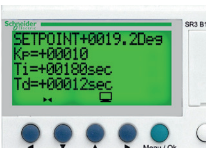
Modifying parameters (Kp, Ti, Td) using the programming and parameter setting buttons
